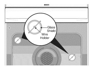
**ACAUTION** Be sure the range is unplugged and all parts are COOL before replacing oven light. Wear a leather-faced glove for protection against possible broken glass.
